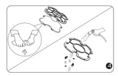
Shake off all debris, and rinse the filter tray with hose water, hand wash the cotton foam.
