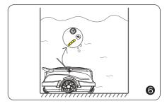
The device will automatically move to stop by the edge of wall when finishing cleaning or battery low.
