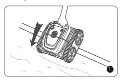
Turn on the device, hold the handle of the cleaner, and put it into the pool vertically.
