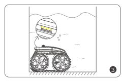
The device will automatically move to stop by the edge of wall when finishing cleaning or battery low.
