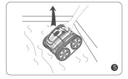
You should take the cleaner out vertically to drain inside water out quickly.
