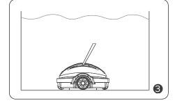
Hold the handle and put it vertically into the pool and fully submerge the device.
