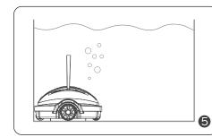
The device will automatically move to stop by the edge of its nearest wall when finishing cleaning or battery low.
