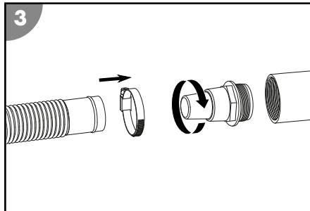
To screw an INTEX swimming pool hose (not included in the package contents) onto the pump or filter vessel, proceed as follows:
