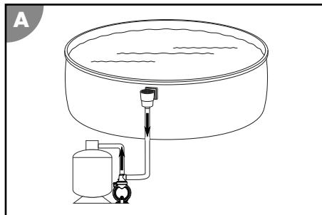
The filter pump pumps the pool water from the pool to the filter system.
