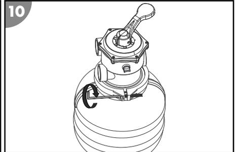
Insert the screws of the locking ring and tighten them clockwise.
